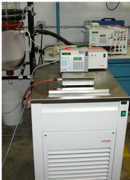
Figure 1: Test Set-up Consisting Mainly of, i) Julabo FP52-SP+HST in the foreground, ii) Ace Glass 30L Reactor in the background on left, and iii) Julabo Messbox Data Acq System in the background on right.
