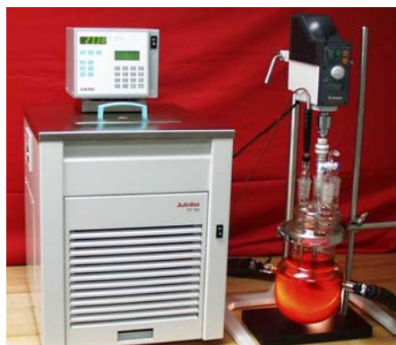
Julabo FP50-HP Benchtop Circulator maintaining temperature in a stirred, Jacketed-Reactor
