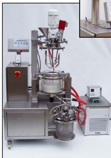
Fig.1.: 'WirelessTEMP' products in an application with an EL- pm -mixer
